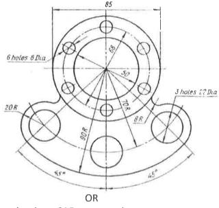
Q.1(B) Draw the given figure using Auto CAD commands
